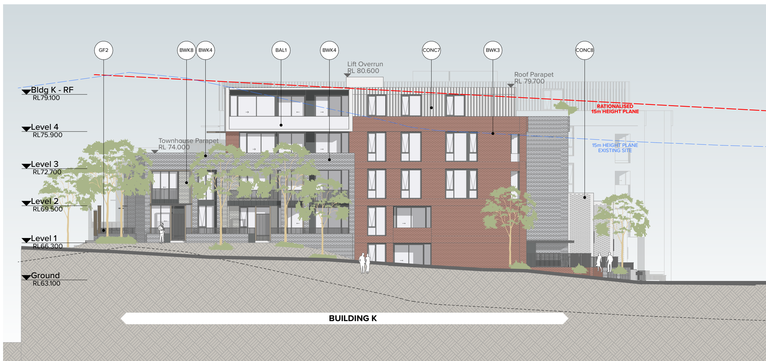
3 - Bldg K East Elevation 1:200
